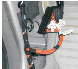
Fig. 4. Distributor location for 164 & 251 bodies (in the left plastic panel)
