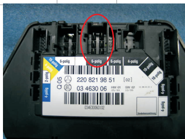
Fig. 2. Seat joystick port that is subject to connection and numeration of its pins
