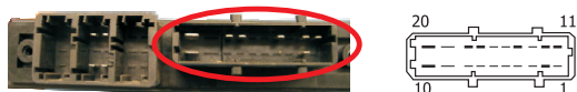
Fig. 4. Fig. 4. Seat control unit connector to which connection is provided and its pin numeration
